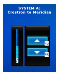
Crestron sends volume up and down commands **VP** and **VM** to the Meridian, using pulses of 0.2s. The Crestron processor and the Meridian are both linked to one another via serial port A.
